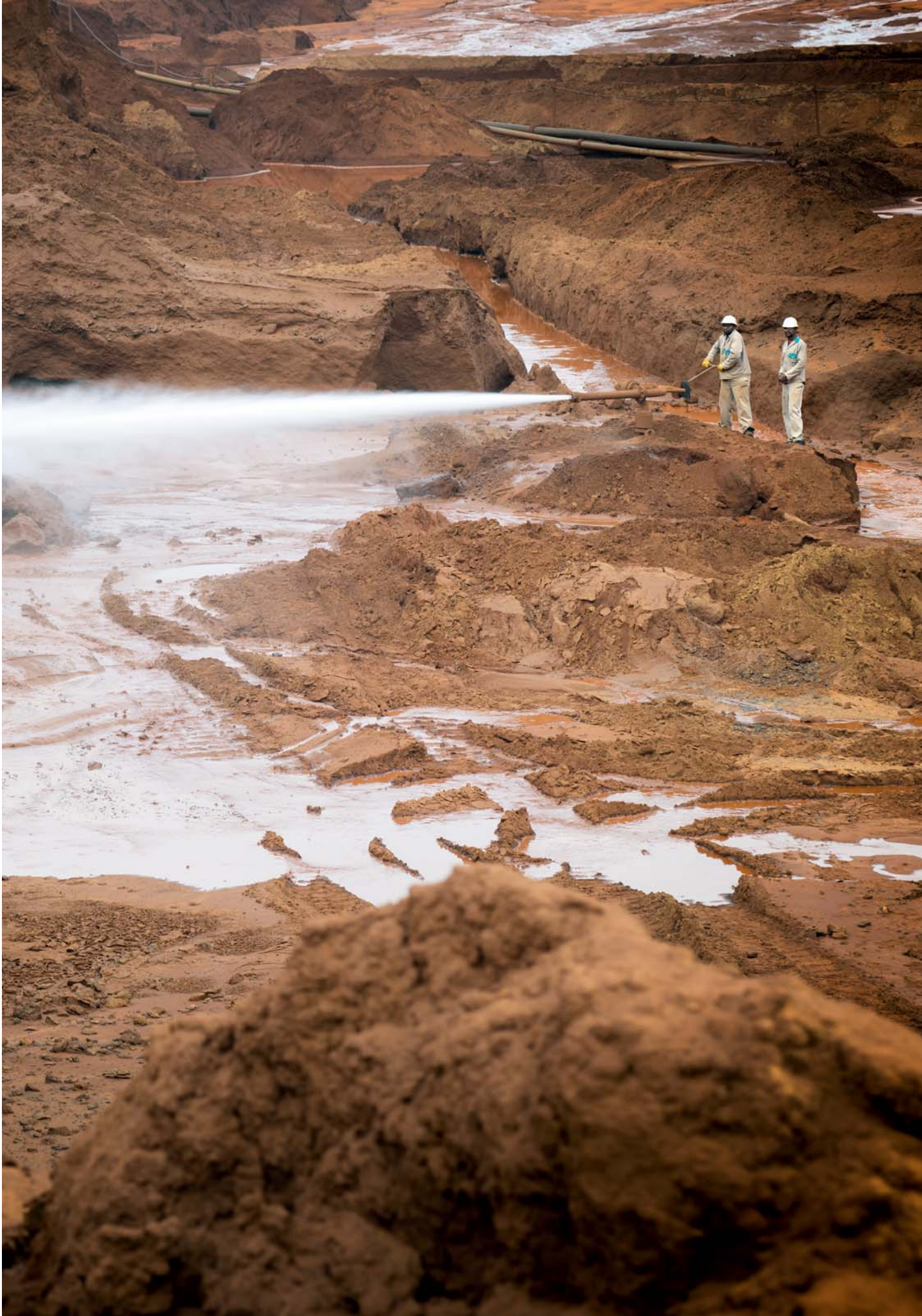
Hydraulic mining at KZN Sands, KwaZulu-Natal. In 2007, it is estimated that Exxaro trained more than 10% of all South Africa's artisans and more than 26% of its mining engineers (Page 122)
