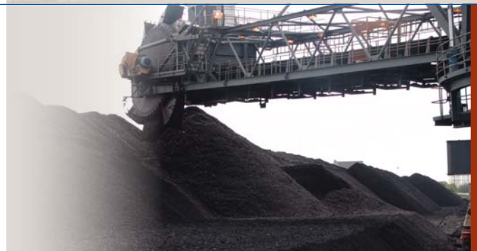
A coal stacker/reclaimer is used for coal handling at the coal stockyard.
